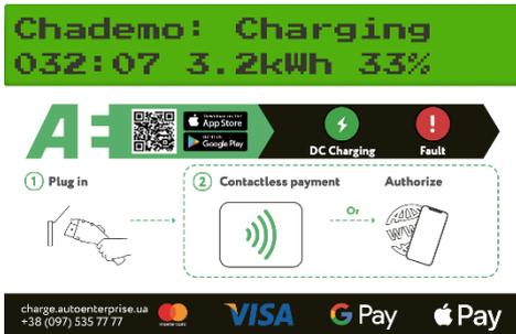
The "DC Output" indicator flashes green quickly when the car is charging in DC Mode "CHAdEMO" / "CCS" / "GB/T DC". In this case the LCD display shows information about charging parameters.
